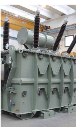
GBE specialises in the design and construction of oil and resin power transformers, with a wide range of solutions. The power reached by the oil transformers is 50 MVA class 145kV BIL 650kV ONAN/ONAF/OFAF 50-60 Hz. while for resin transformers the power reaches 30MVA in class 52kV BIL250kV,
