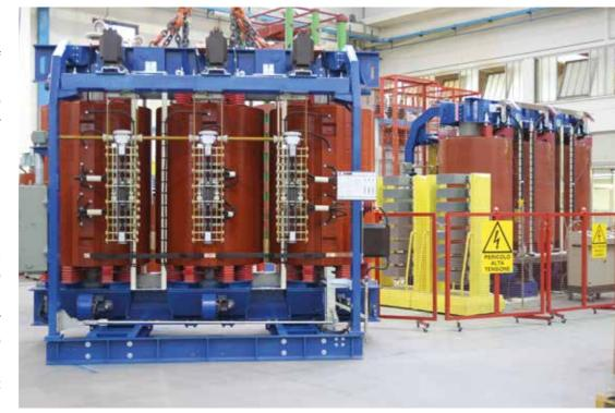
A result that is all the more significant considering that the design, manufacture and supply were performed in record time: 8 x 35 ton transformers were made in less than 12 weeks, including the verification of their resistance to short circuit at a certified SIEMENS laboratory. A great demonstration of dynamism and speed of response, made possible by the contribution of the new GBE plant, entirely dedicated to steelworks.
