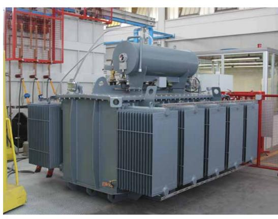
Oil-immersed short-circuit limiting reactor with shield, 4800 kVAR, 11kV
