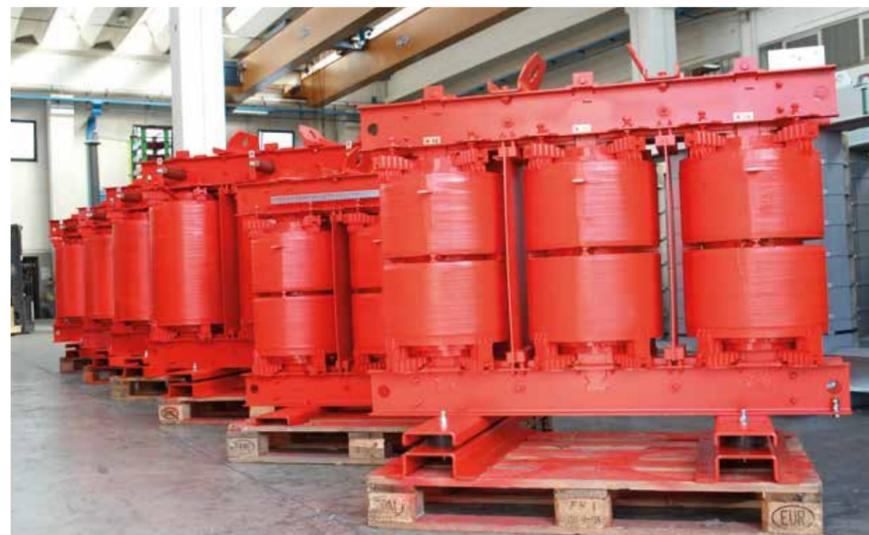
If reliability is the first requirement for an electricity distribution network, it is all the more reason for installations in places where access is difficult or where there is no on-site support structure. So that makes all the more significant GBE's supply of 77 detuning reactors, with reactor power from 200 kVAR to 1000 kVAR, for a special project in Africa in collaboration with a leading manufacturer of capacitors in Mantua.
