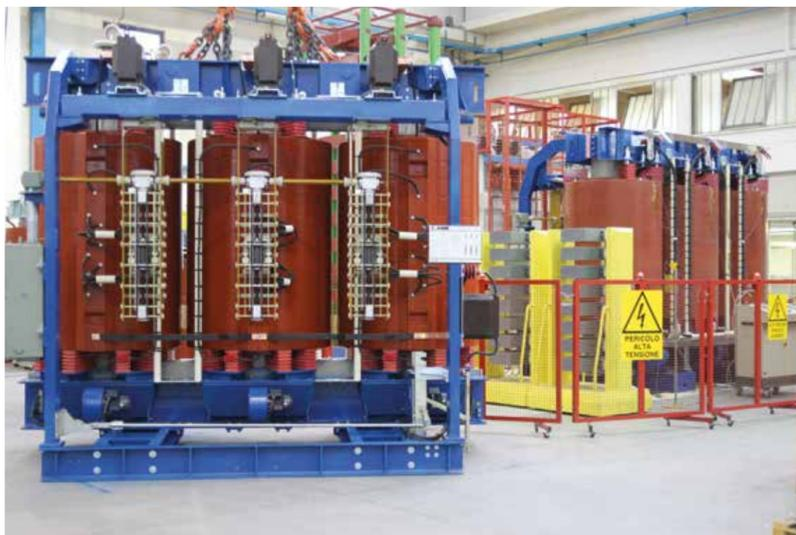
After having successfully satisfied this first complex request, the request then came for a further supply, in which among the specifications, in addition to the limitation of noise emissions, were also restrictions on the dimensions, in order to install the transformers within existing sub-stations. Even this requirement has been fully satisfied, thus confirming GBE's expertise in the area of special projects, to satisfy any performance and installation demand of the Client.
