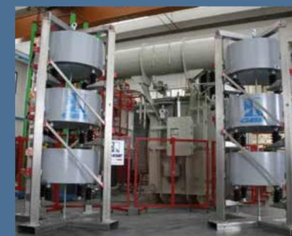
Alongside the production of reactors, GBE distinguishes itself through the completeness and variety of its range, with class F or H air and resin and oil insulated machines, for indoor and outdoor applications up to 5000 A/52 kV.
