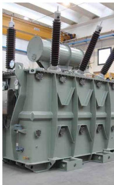
GBE specialises in the design and construction of oil and resin power transformers, with a wide range of solutions. The power reached by the oil transformers is 50 MVA class 145kV BIL 650kV ONAN/ONAF/OFAF 50-60 Hz, while for resin transformers the power reaches 30MVA in class 52kV BIL250kV, AN/AF 50-60 Hz.
