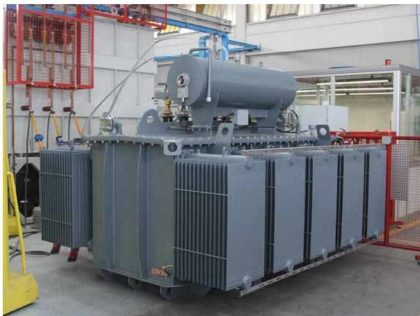
Oil-immersed short-circuit limiting reactor with shield, 4800 kVAR, 11kV
