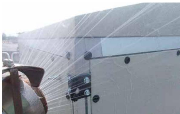
Seal testing at the TÜV Laboratory (Italy)
